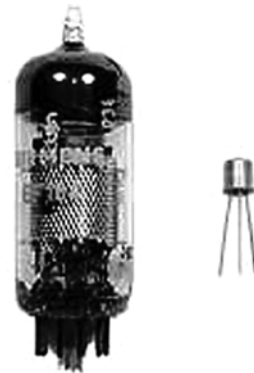
FIGURE 12-32 The Vacuum Tube vs. the Transistor
