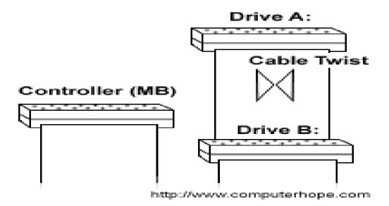
A standard floppy drive connector contains 34-pin wholes we have listed the pins and the description of each pin below.
