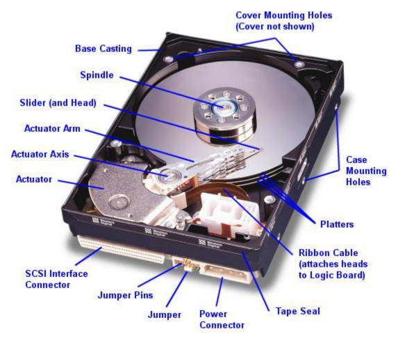
Hard disk drives are almost as amazing as microprocessors in terms of the technology they use and how much progress they have made in terms of capacity, speed, and price in the last 20 years. The first PC hard disks had a capacity of 10 megabytes and a cost of over \$100 per MB. Modern hard disks
