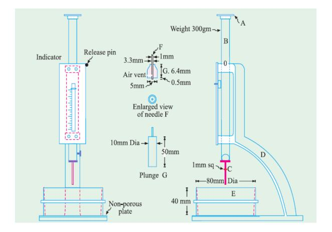
**Objective:** To determine the initial and final setting time of a given sample of cement.
