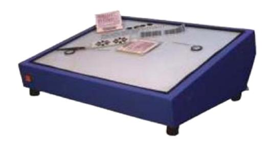
The PCB Drafting Kit includes Various tapes, pad and other material for making PCB Artworks.
