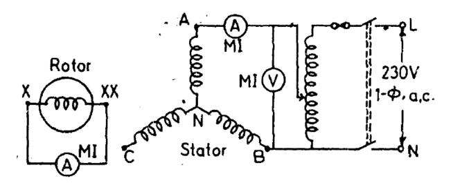
1. Let the applied voltage across the terminals A,B of the stator winding with terminal C kept isolated be E volts and the current flowing through the winding in currentbe I amperes. The ration of voltage across each phase to current is a reactance which can be represented by a quantity A' i.e.
