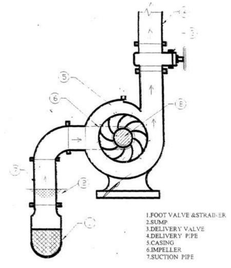
Fig. Component parts of Centrifugal Pump
