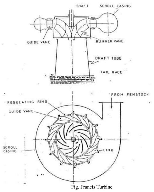
Tools required: Francis Turbine, Pressure gauges, Tachometer and
